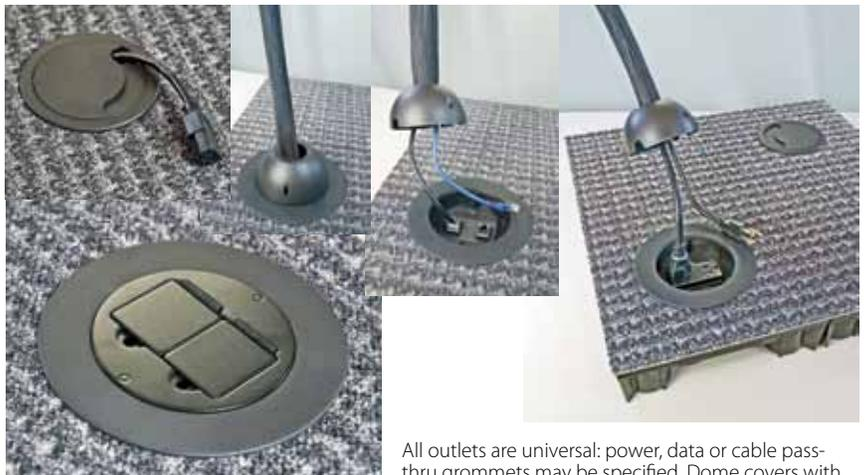
All outlets are universal: power, data or cable pass-thru grommets may be specified. Dome covers with flexible conduit provide an uncluttered harness to the furniture. These replace the standard, hinged covers. RJ45 data connections are standard. Specify custom connectors as required.
