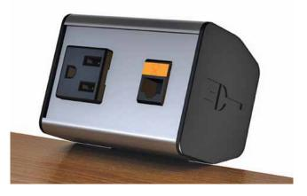
The Seclusion can be mounted under the table or on top according to the users' convenience. Seven standard configuations provide power only, or power and data RJ45 cat 6 connectors. Wiring for Circuit 1 and Circuit 2 and four Daisy-T Cable lengths are available. The Daisy-T cable connects the Seclusion to the Daisy-T Power Manager. The length required is based on the placement of the Daisy-T.
