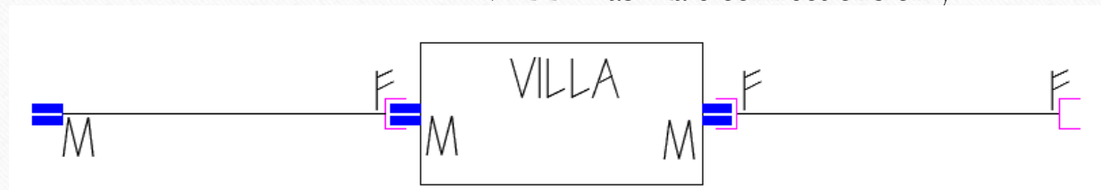
Villa connections on both ends – require a cable that has a FEMALE connection on both sides. The VILLA has Male connections only.
