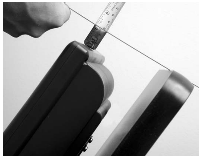
Choosing correct placement of the VESA Mounting Assembly should result in proper clearance of the LCD display. The LCD housing should have 1/2 inch to 1 inch clearance between the edge of the flipIT top and the LCD housing. After completing the next step, trial fit the LCD and see if you need to choose different mounting holes.
