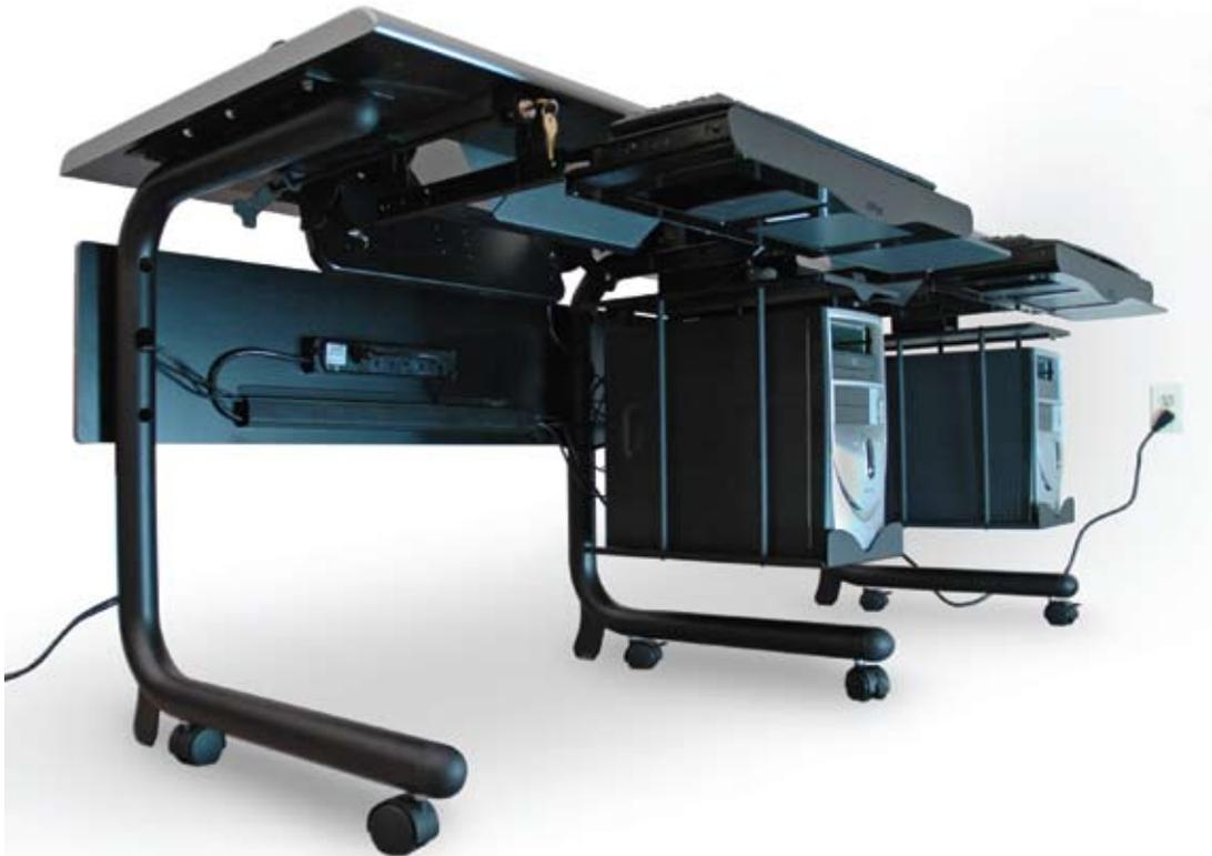
Data wire management passes cables through the leg from the floor to the modesty panel. J-channel conducts the cables horizontally. A power strip or surge suppressor with 10 foot cord is provided for power distribution. The back of the CPU is open for connections. Keyboard, mouse and screen are easily connected. No mess. Shown with Brig CPU holders, FIK-18 flipIT® for LCDs up to 17.5" wide, and locking casters for mobility. Other options available, including the flipIT® Laptop Safe
