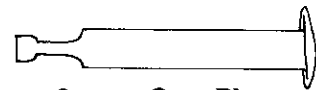
8 ea. - Cam Pins push through holes in panels. (Back Panel, Support Panels)
