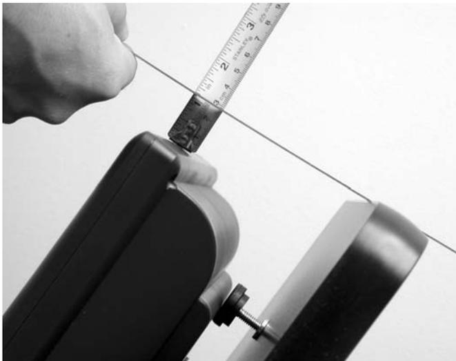
Factory placement of the VESA Mounting Assembly should result in proper clearance of the LCD display. The LCD housing should have 1/2 inch to 1 inch clearance between the edge of the flipIT top and the LCD housing.
