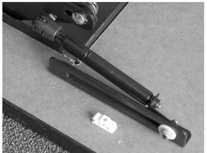
Damper Anchor Assembly mounted to desktop.
