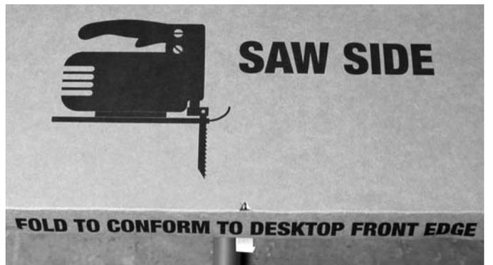
Position template face up on the desktop marked **TEMPLATE FOR TOP CUT-OUT: SAW SIDE**. Fold the tab section of the template and place it against the front edge of the desktop surface. Locate the template's centerline notch to the centerline you marked on the edge. Tape template to the surface to secure in position.
