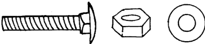
*16 ea. - 1 1/2" Caster Bolts, Nuts & Washers for Caster Plate top
