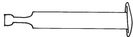
12 ea. - Cam Pins push through holes in panels. (Side, Back, and Bottom Panels)
