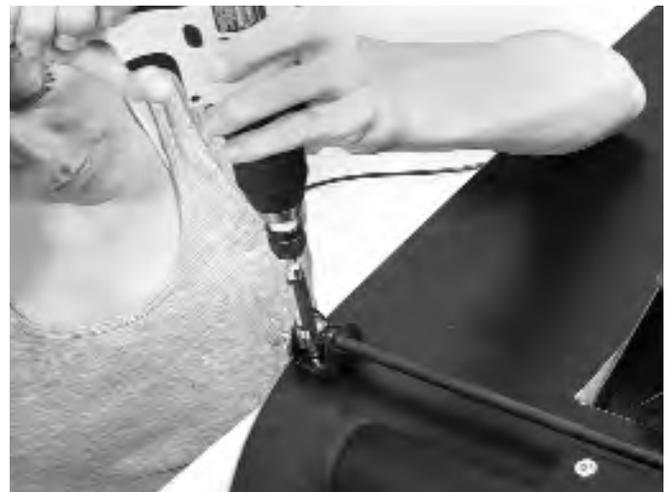
Hold the bracket in position and mark the location for drilling pilot holes. Drill precise pilot holes using 1/8" drill and depth gauge. Install using 2 Phillips 5/8" wood screws.
