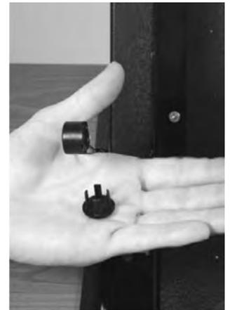
Using a slot screwdriver blade, pry the locking cap off completely and set it aside.
