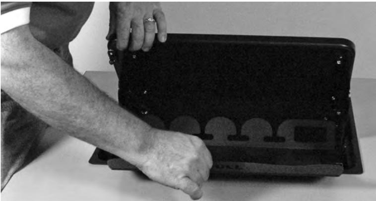
PULL the tray out, and gently assist by pulling the top lid. When the gas spring is later installed, the assist is not required.
