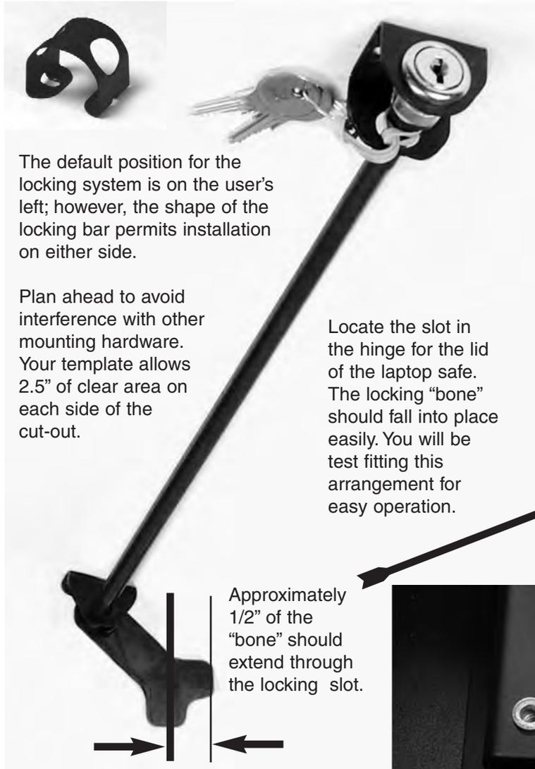
The default position for the locking system is on the user's left; however, the shape of the locking bar permits installation on either side.
