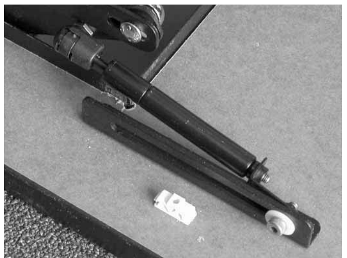
Damper Anchor Assembly mounted to desktop.
