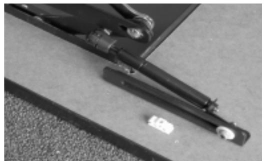
Photo shows Damper Anchor Assembly mounted to desktop.
