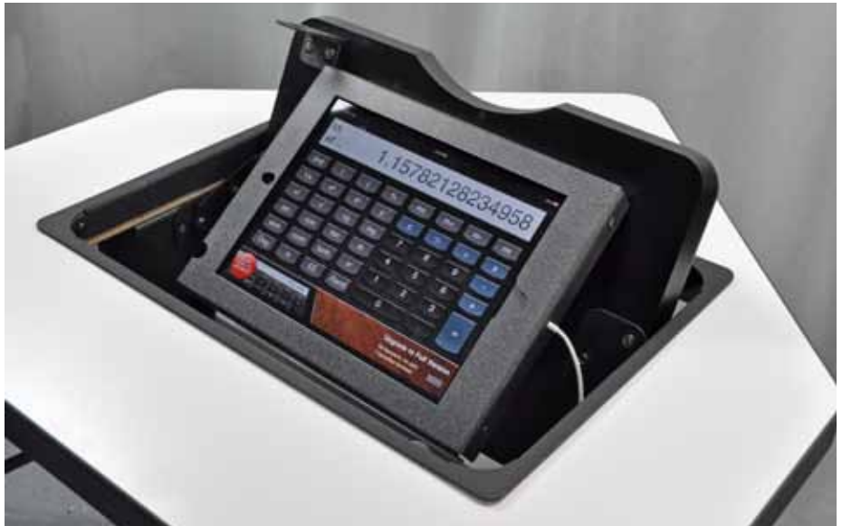
The NO HOME BUTTON lock out tab is optional. If desired, capture the tabs and hold in place as shown before closing the flipIT enclosure.
