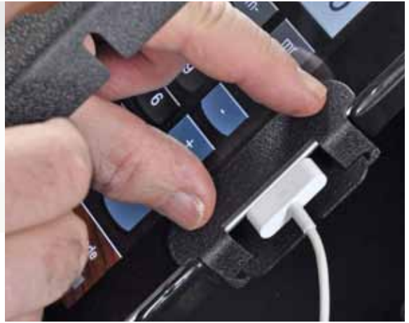
The NO HOME BUTTON lock out tab is optional. If desired, capture the tabs and hold in place as shown before closing the flipIT enclosure.
