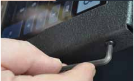
The NO HOME BUTTON lock out tab is optional. If desired, capture the tabs and hold in place as shown before closing the flipIT enclosure.
